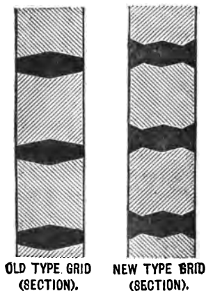
Fig. 19.—Grids (greatly magnified).
